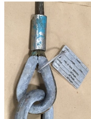
Figure 1: Fitting has a uniform appearance
