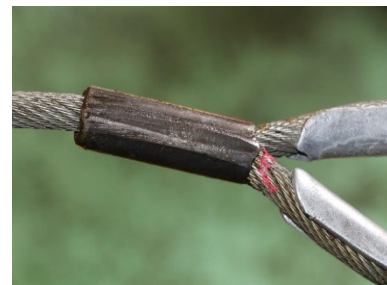
Figure 3: Fitting is deformed with "ridges" of extra material present from over-crimping.
